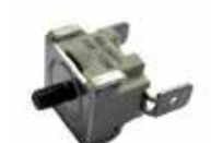
9V068 TERMOSTATINO 180° CERAMICA M4X6 RIARMO AUTOMATICO TERMOSTATINO 180° CERAMIC M4X6 AUTOMATIC RESET
